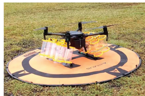
A drone with canisters built to release biocontrol agents onto invasive strawberry guava.
